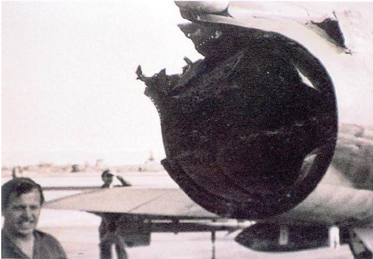
Damaged Mirage III CZ tail as a result of a direct SA – 7 hit
