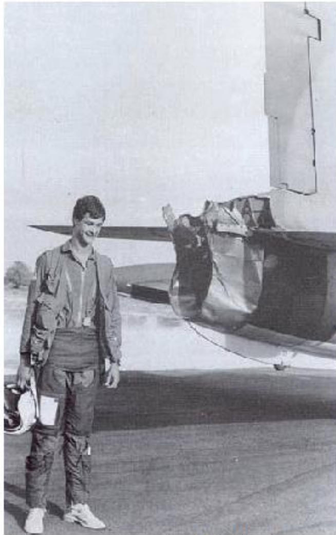
Damaged Impala Mk II jet pipe as a result of direct SA -7/14 hit
