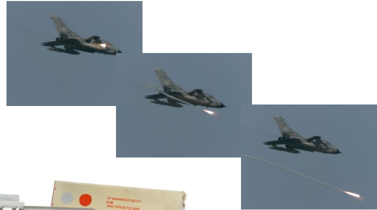
No. 218 K7 Type 1 propelled flare
