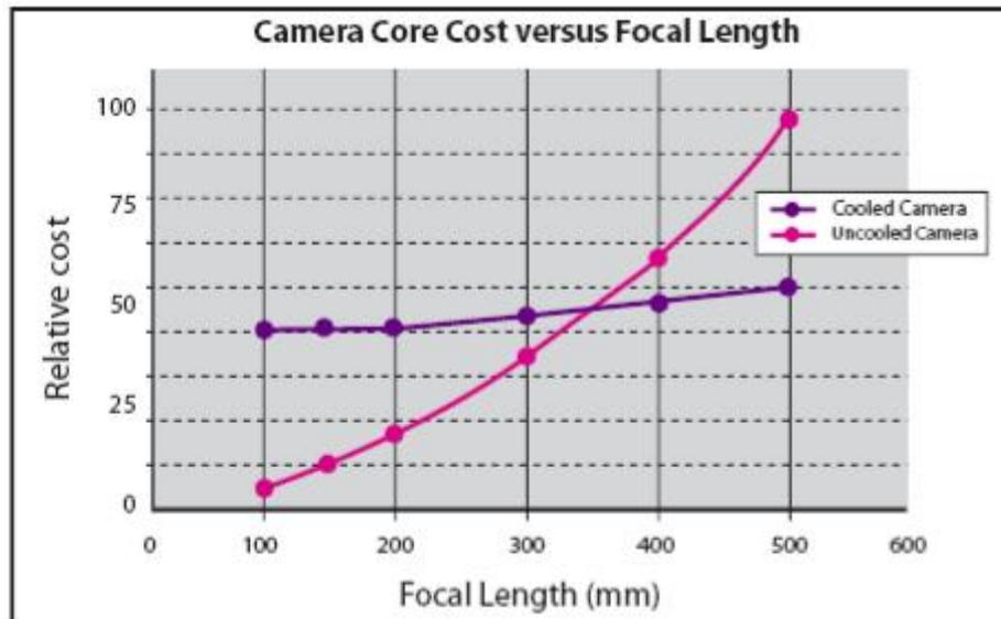
*Relative camera cost of cooled and un-cooled IR systems as function of lens focal length*
