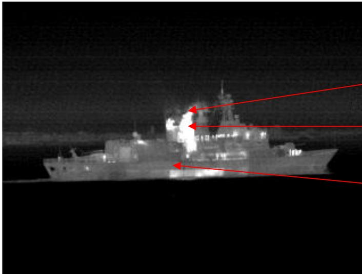
Exhaust plume (emission by hot exhaust gas molecules)
