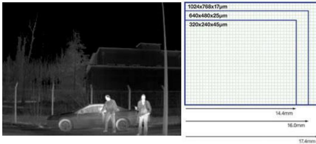
*IR image captured with 1024x768 un-cooled a-Si FPA (ULIS) and illustration of nearly constant sensor size even as array density increase (right).*
