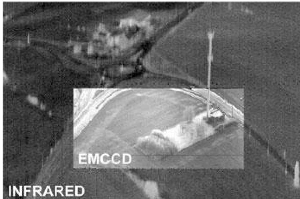
Example fused image comparing EMCCD with infrared under starlight conditions
