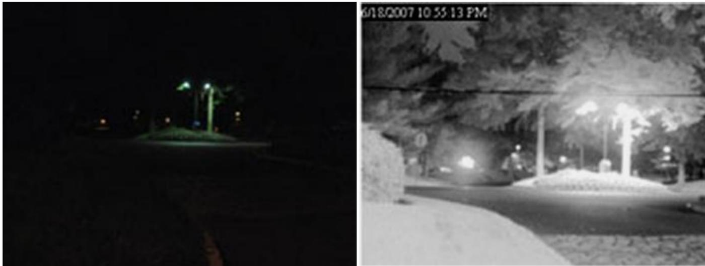
*A parking lot at night with a normal VIS (left) and special InGaAs SWIR camera (right).*
