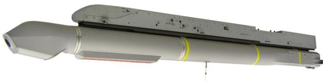
BOH provides covert sustainable pre-emptive dispensing, missile warning, forward firing of flares and cocktail dispensing. All these capabilities have been incorporated into the form-factor of a missile utilizing the well established AIM-9 Sidewinder and AIM-120 AMRAAM interfaces and characteristics for lean aircraft integration.
